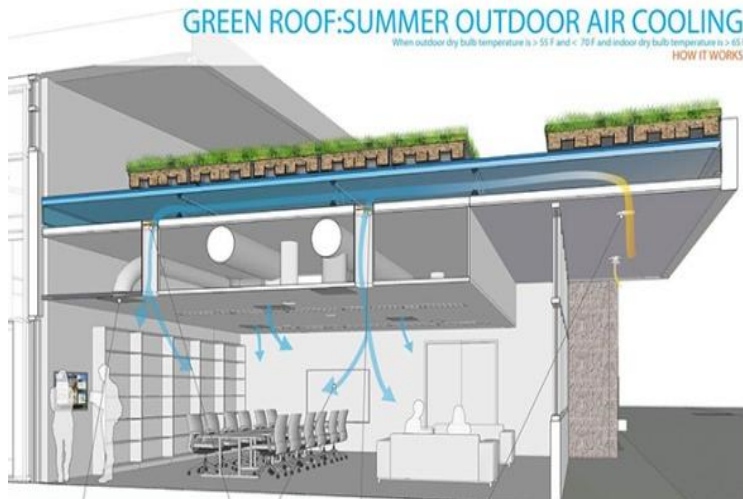
Active green roof. Fuente: climate colab.
